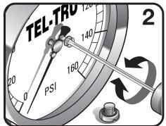
**Insert** a *small* bladed screwdriver into the hole in the lens. **Correct** the pointer position by adjusting the screw on the pointer. If the screw can not be reached, temporarily remove the lens to allow access. Then re-assemble gauge.
