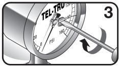
**Replace** screw in lens using a *large* bladed screwdriver.
